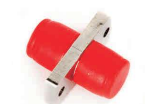
Part Number Description A-F-F-U-S- CF-Z-M-M-5 Mating sleeve adaptor, FC & FC connecting port, simplex, rectangle shape, zirconia internal tube, metal material
