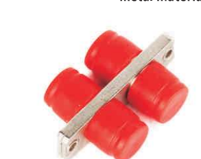
Part Number Description A-F-F-U-S- CF-Z-M-M-5 Mating sleeve adaptor, FC & FC connecting port, simplex, rectangle shape, zirconia internal tube, metal material
