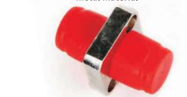
Part Number Description A-F-F-U-S- FX-Z-M-M-5 Mating sleeve adaptor, FC & FC connecting port, simplex, square shape, zirconia internal tube, metal material
